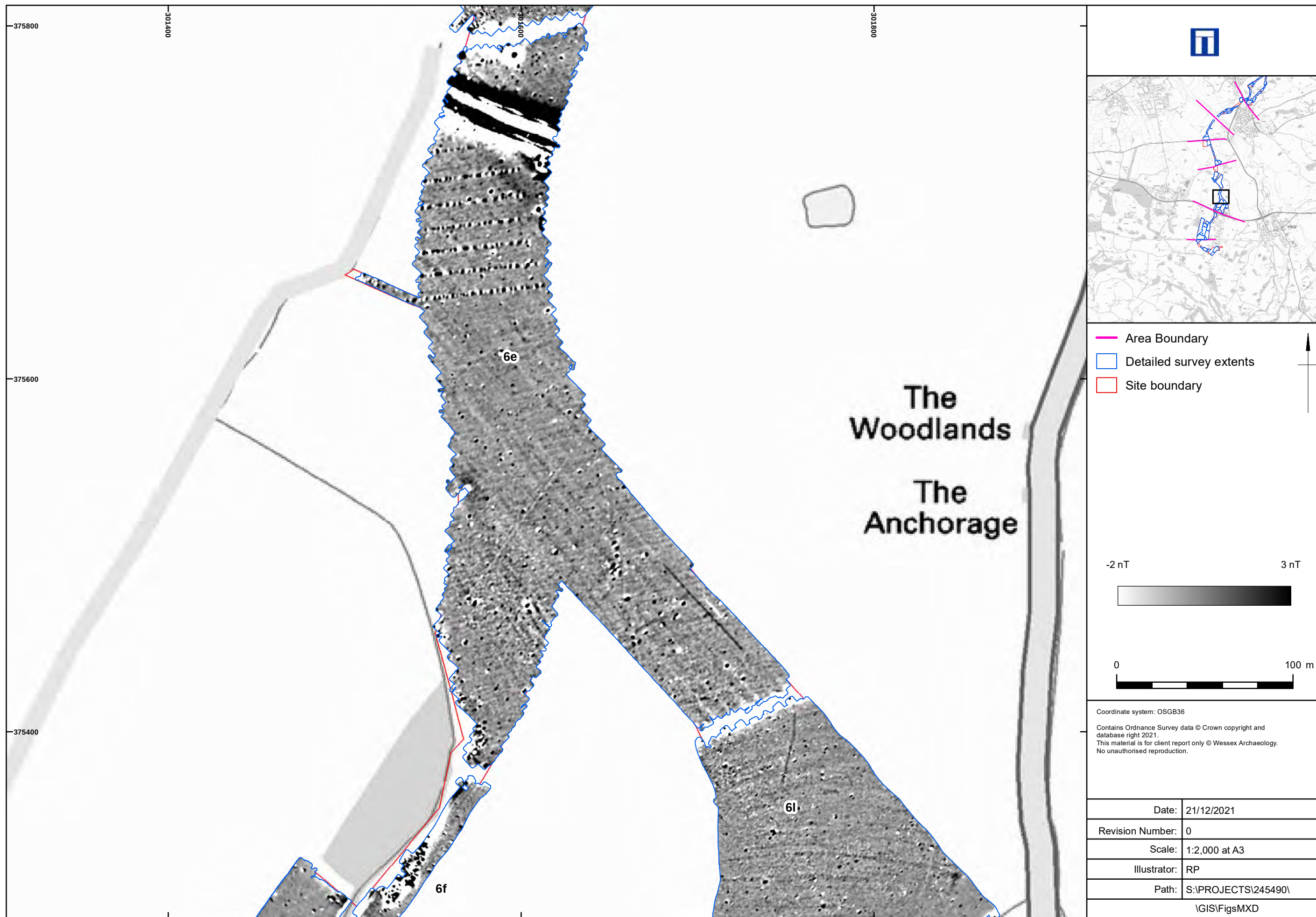
Detailed gradiometer survey results: greyscale plot Area 6 (centre/south)
